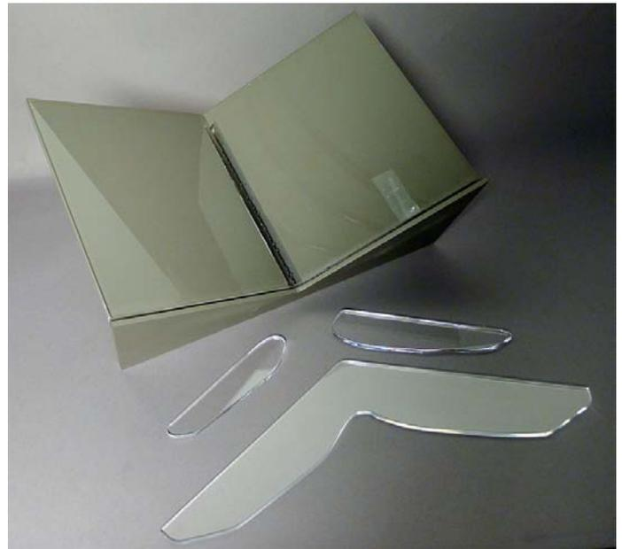
Figure 3: Painted acrylic design cradle with separate clear-acrylic boomerang-shaped foot piece (ledge) that fits into groove on cradle and separate packing pieces for text block support. This style cradle is used for rotations of manuscripts from the permanent collection.
