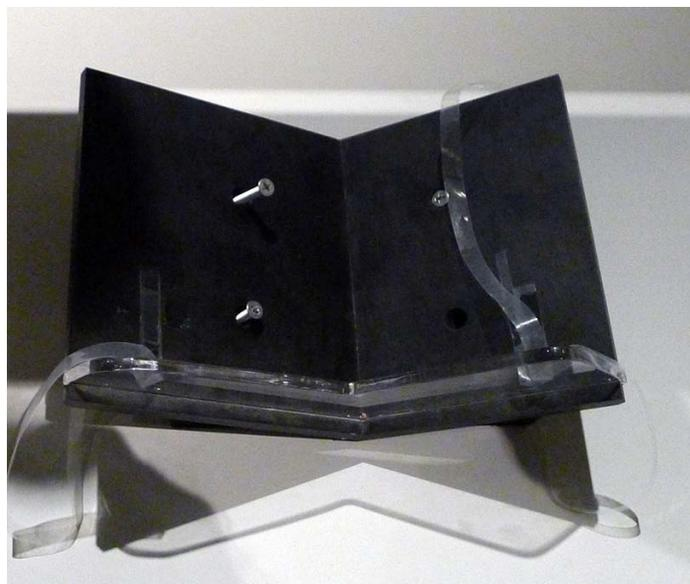
Figure 8: Assembly of foam-based, pieced design cradle for use in loan exhibitions. Black acrylic sides (either separate or welded with acrylic adhesive at V-join) are screwed to foam base of cradle. Clear acrylic boomerang-shaped foot piece (ledge) is inserted into grooved lower edge. Manuscript is strapped with polyethylene strapping taped to the acrylic sides of the cradle.
